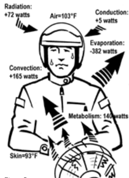
Figure 5 Heat Balance Wearing a Vented-Windproof Suit With 103°F Air Temperature Required Evaporation: 19 oz. per hour
