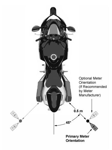
Figure 1 Orientation of Sound Level Meter During Testing
